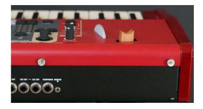
3. When you get to your gig, remove the thumb screws, place the plate on top of the Stage 2, and replace the thumb screws. Verify the alignment of the plate by making sure it's not touching the mod wheel, then tighten the screws.
